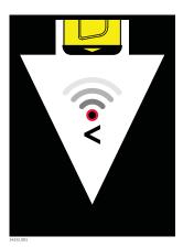
This screen indicates that the signal source is too low to provide a depth reading.
