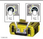
To indicate that the tracing signal reaches a good level, the Power Output LED indicator and the audible tone change from pulsed to continuous.
