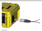
3. Connect the red cable to the positive (+) terminal on the trace rod. Connect the black cable to the negative (-) terminal.
