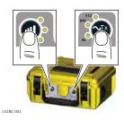
3. Place the transmitter over the utility with the arrows running in line with the suspected direction of the utility.
