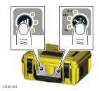
7. Set the locator to Signal Transmitter mode and select the required frequency.
