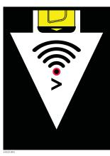
This screen indicates that the signal source is too high to provide a depth reading.
