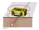
4. Set the locator to Signal Transmitter mode and select the required frequency.
