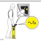
7. At a distance of 5 m (16 ft) to the connection point, circle around the connection point.
