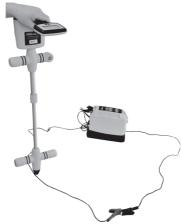
**Configuration for Testing the Conductive Attachment**
