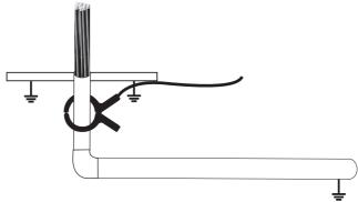
Inductive coupling with the signal clamp
