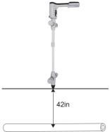
Press and release the DEPTH BUTTON on the handle of the receiver. Within seconds, the digital display will show the depth of the conductor in inches or centimeters, depending on the instrument version.
