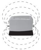
Signal Field Generated by Transmitter when in Inductive Use
