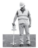
Position of Receiver for Tracing
