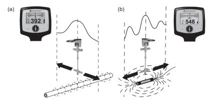
Due to this construction, the Sonde gives a different "Peak" pattern (see diagram b) — note that there are three distinct peaks — a small peak — a large peak — a small peak. The Sonde is located under the center of the "large peak," when locating across the direction of the Sonde, it provides the normal peak response. Note also that the Sonde Direction Indicator points across the line of the Sonde when the receiver is directly over it.
