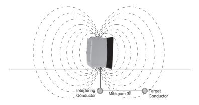
Position the transmitter for minimum interference
