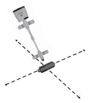
When over the Sonde, press the On/Off button once to display the depth reading.
