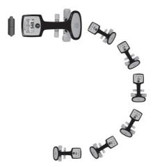
To pinpoint the Sonde, find the maximum numerical signal strength in both directions.
